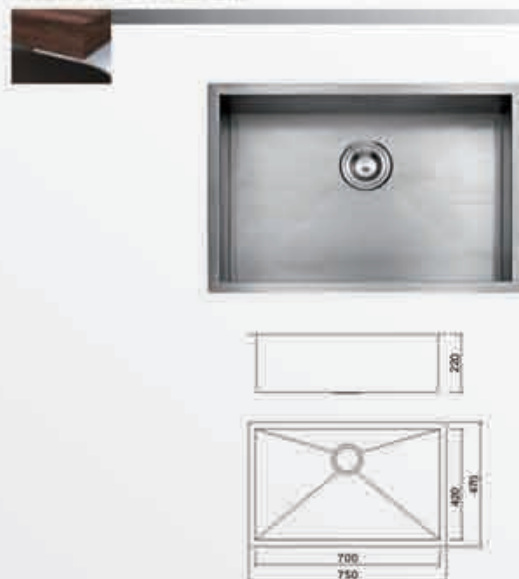
Model: DC-S754 Size: 750x470mm Depth: 220mm Surface: Satin Thickness: 1.2mm Material: SUS304#
