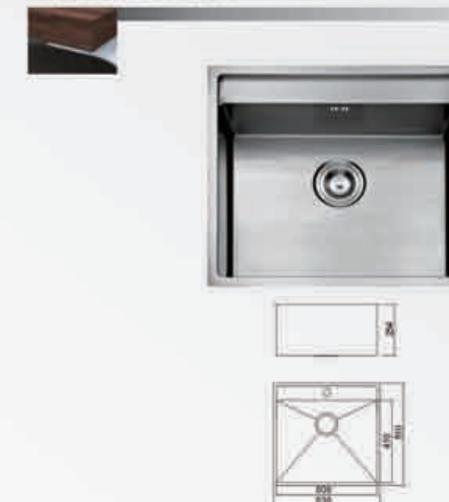
Model: DC-SR535 Size: 530x510mm Depth: 254mm Surface: Satin Thickness: 1.2mm Material: SUS304#
