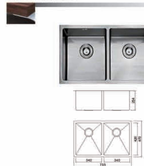
Model: DC-SR754 Size: 755x470mm Depth: 254mm Surface: Satin Thickness: 1.2mm Material: SUS304#
